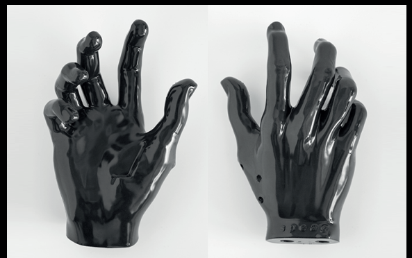
SHO3TO110 hand phantoms with CTIA-compliant handgrips for 5G OTA applications
